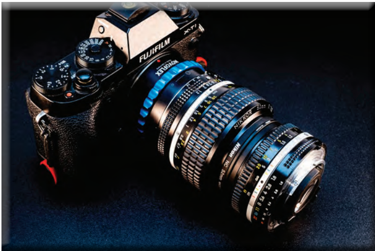
A Nikon 50mm f/1.8 manual lens is coupled to the Nikon 50mm f/1.2 lens on a FUJIFILM X-T1 with a Novoflex adapter.
