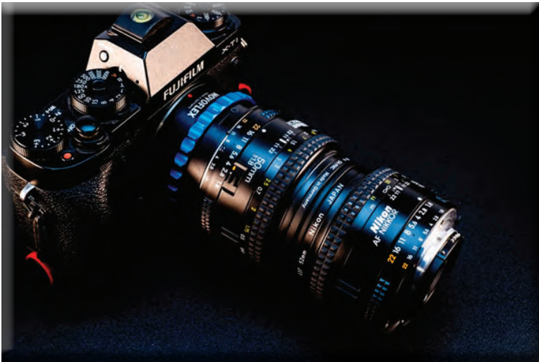
Two Nikon AF 50mm f/1.8 lenses are coupled on a FUJIFILM X-T1. This setup gives you a 1:1 magnification for macro work.
